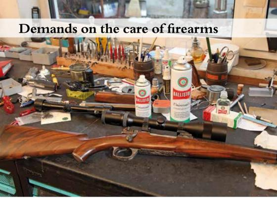
When firing a shot there are Temperatures of several hundred degrees centigrade and acid combustion gases under a pressure of up to 500 atmospheres, which provides the bullet with the necessary initial acceleration. These extreme conditions in the barrel foster wear and tear and corrosion extremely. On top of that all kinds of weather affect the outside of the weapon.
